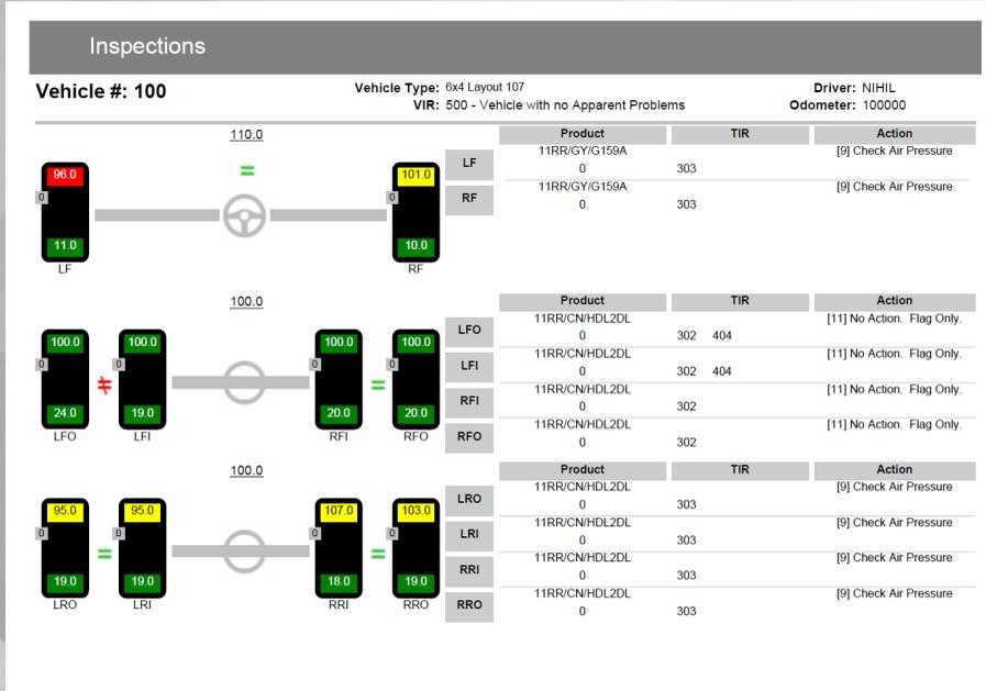
The Vehicle Inspection Report shows a footprint of the vehicle and instantly color coordinates the tires based on fleet parameters.
